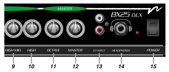
**13. CD INPUT:** Use these RCA jacks to connect the line level (or headphones) output of a CD player, tape deck or rhythm machine to the amplifier. The signal level from these jacks is adjusted by the Master control (#12). If the signal from the source connected to these jacks is too strong, use the output level control on the source to adjust the signal to obtain the proper level for a good mix.
